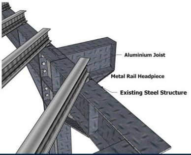
When laying the rails/joists onto existing steel substructure it is recommended to use our Rail Headpiece, which is secured to the substructure at any angle required. This also provides effective barrier protection between the two metals.
