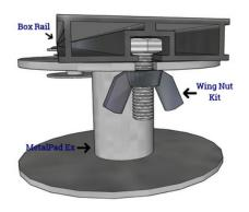
Utilising our MetalPad Ex Class A Fire Rated Pedestals with the M8 Wing Nut, which can be tightened by hand, offers significant benefits. This approach allows for the initial loose placement of pedestals and joists for precise positioning. Once in place, you can then securely tighten them to establish a stable and robust substructure system.
